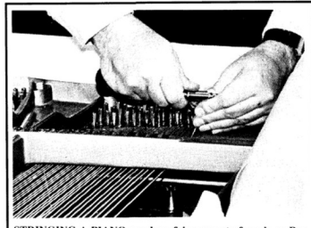
STRINGING A PIANO can be a fair amount of work, as Ray Citak well knows. Here, he wraps the string around the tuning peg, which gets hard to do with the bass strings.
