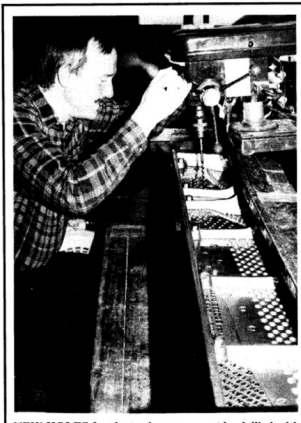
NEW HOLES for the tuning pegs must be drilled with precision. Steve Westfahl must get the exact angle and size for each hole, as he drills.
